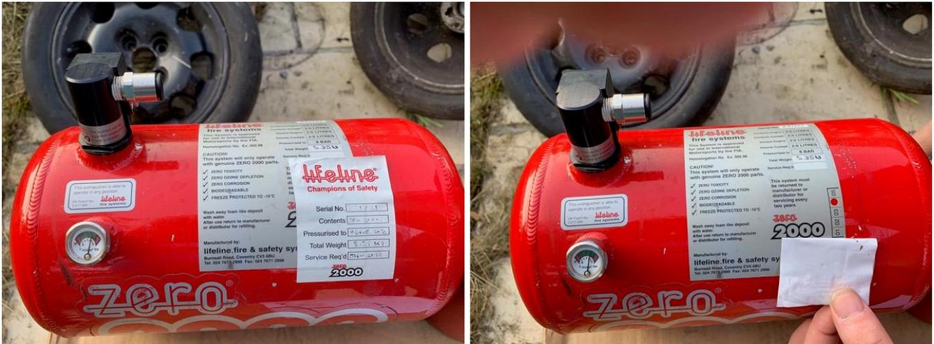
The second example appears to show two genuine and serviceable bottles, with gauges showing in the green, but one had been discharged and was 1kg lighter! If in doubt you can request to weigh the bottle (the service weight should be on the service label). This shows that on occasion gauges can get stuck or blocked up and not give a true reading, or of course they could be deliberately manipulated to show a false reading, and in this case weight is the best indicator.
