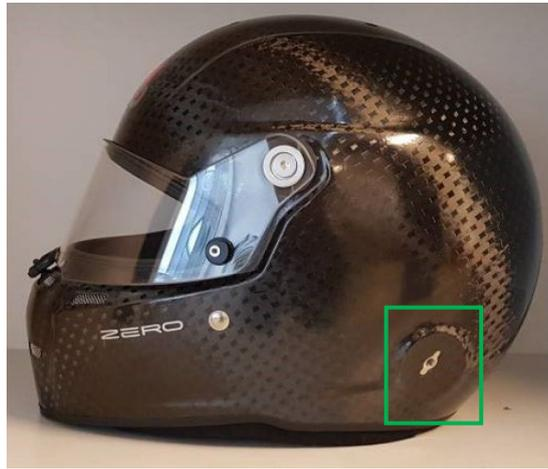
*Fig.2b - Helmet-M6-anchorage removed*
