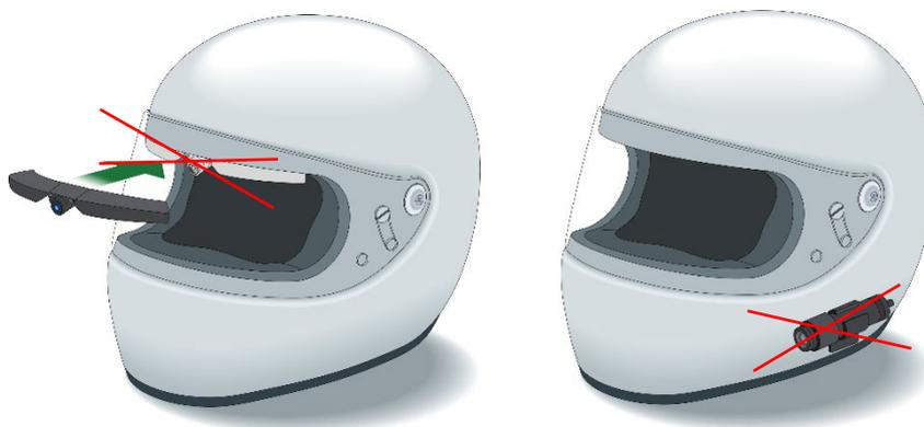
*Fig.1 – NOT approved helmet camera installation*
